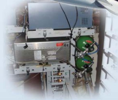
In CARIBIC, a cargo container is deployed as a flying laboratory aboard one aircraft. A special multi-functional inlet system allows optical measurements and accurate sampling for aerosol and trace gases.
